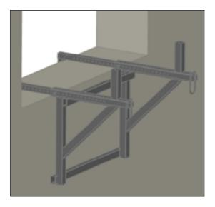
2. Attach the winch and lower the crossbar. Ensure tension in the winch rope by attaching additional load.
